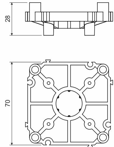
product description: use the support to fix the boxes between the formwork walls
