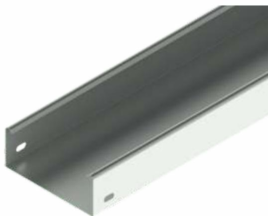
product description: Cable tray is designed to create a cable route. The joining of the trays is performed by using of the couplings NIXS and by the bolts NIXSM 6X10. The tray is connected to the accessory directly, with no couplings; the tray is inserted into the accessory. Fasten using NIXSM 6X10 bolts.
