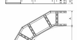
product description: The horizontal bend is used to bend cable trays running through cable ladders by 90° in a horizontal direction.
