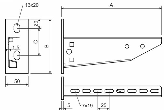
surface finish: F - Hot Dip Galvanized, zinc-layer 55 µm (min. 45 µm)
